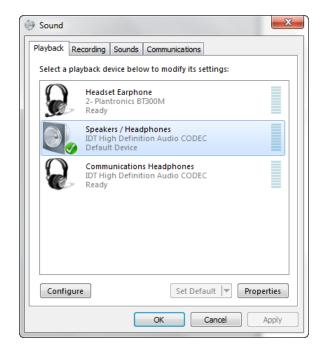
In this example, the user has a Plantronics BT300M (the USB dongle accompanying a Voyager Legend UC) connected to their PC.
